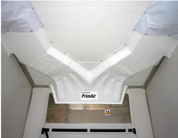
The PrimAir Split Air Chute System is designed to provide uniform temperature throughout the entire trailer. The unique diverter evenly distributes air to each side chute, which then guides the air to the rear of the trailer.
