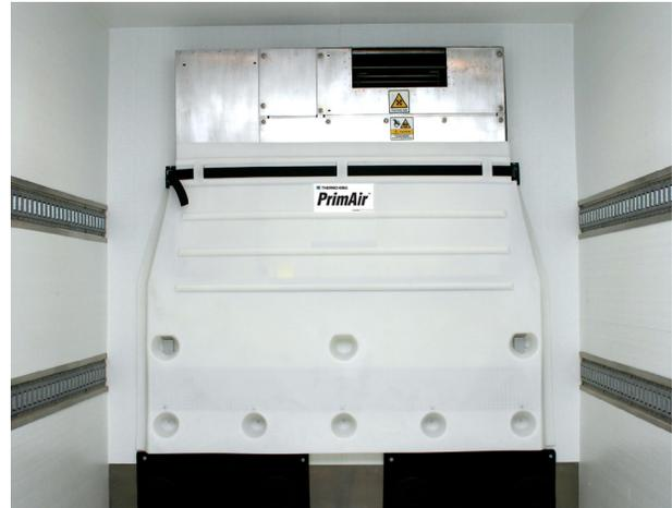
Reduce short-cycling and maintain uniform product temperatures with this easy-to-use bulkhead. It takes less than one minute to remove the bulkhead to access the refrigeration unit. Replace pallet stops as needed without replacing entire bulkhead. No tools needed.
