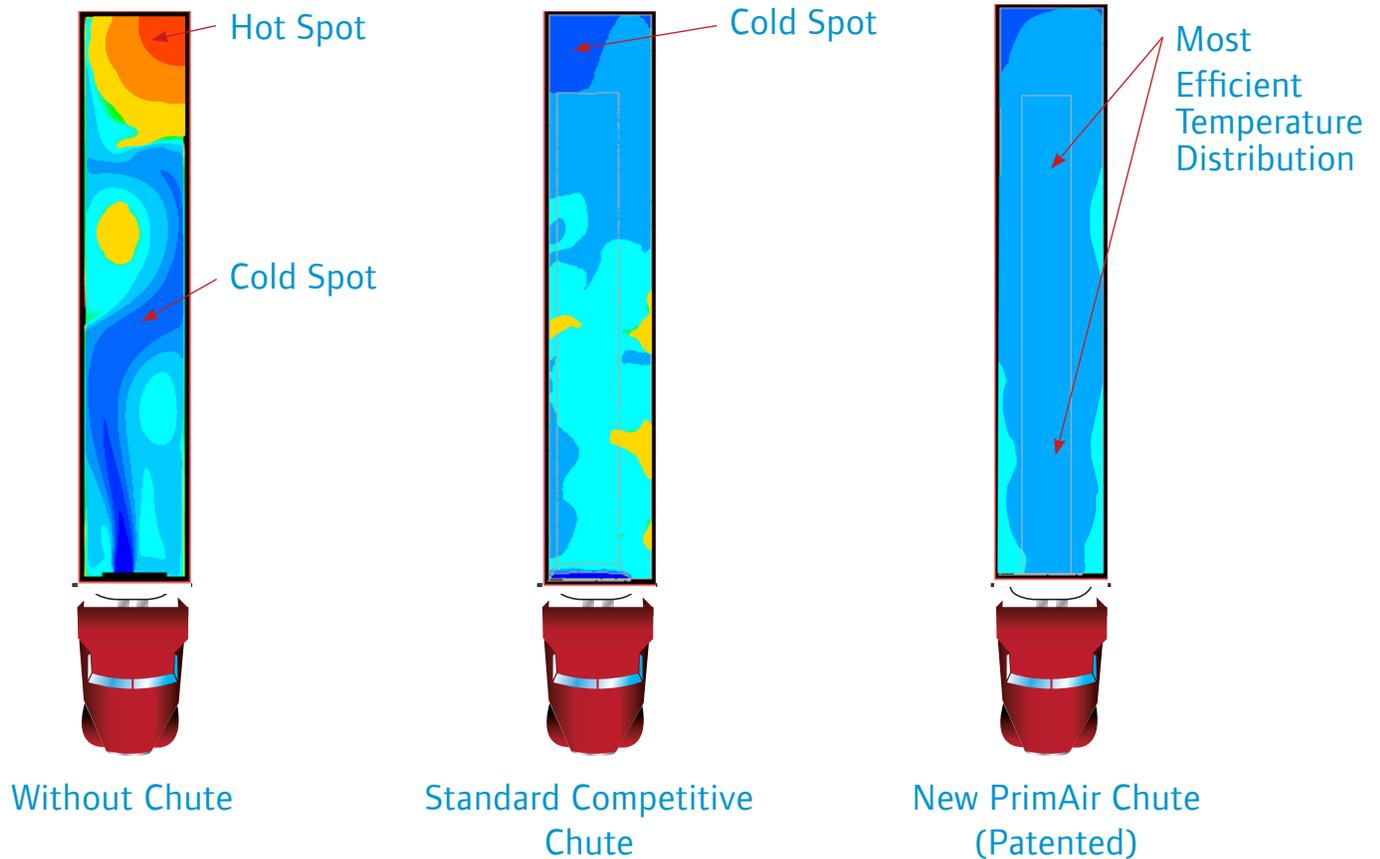
*Results based on Thermo King CFD analysis on loaded trailer.*
