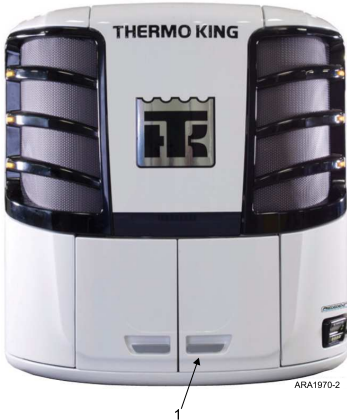
Figure 8. Door Latch Location
