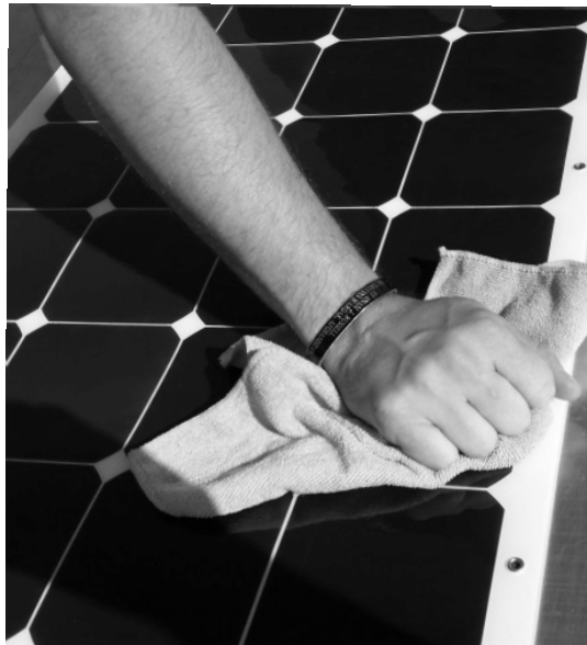
Figure 5. Firmly press panel down over entire area
