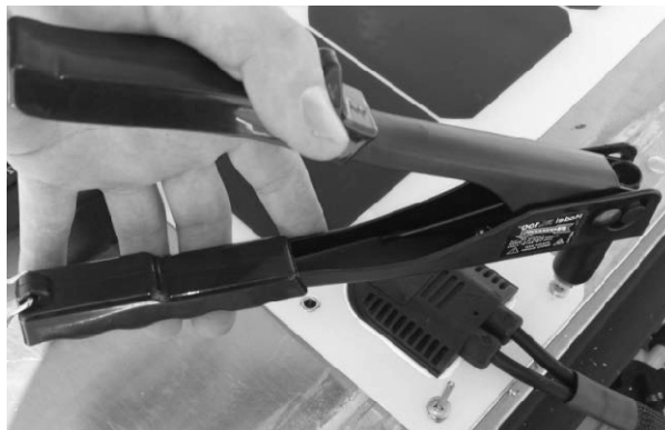
Figure 5. Fastening panel using rivets shown
