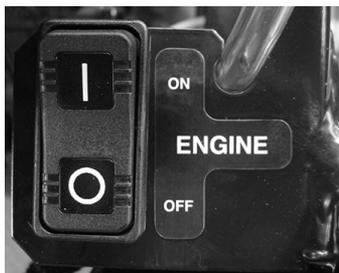
The APU Engine On/Off Switch functions as a service switch. It allows maintenance personnel to disable the APU engine. This assures the engine will not crank even if the HMI On/Off button is pressed on.
